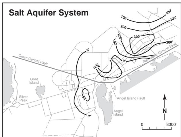
**Figure 5. Isopachs of the Lower Gravel Aquifer, Lower Aquifer System, Main Ash Aquifer, Marginal Gravel Aquifer, Tufa Aquifer, and Salt Aquifer System (thickness in feet, superimposed on outlines of brine ponds and pertinent fault systems).**
